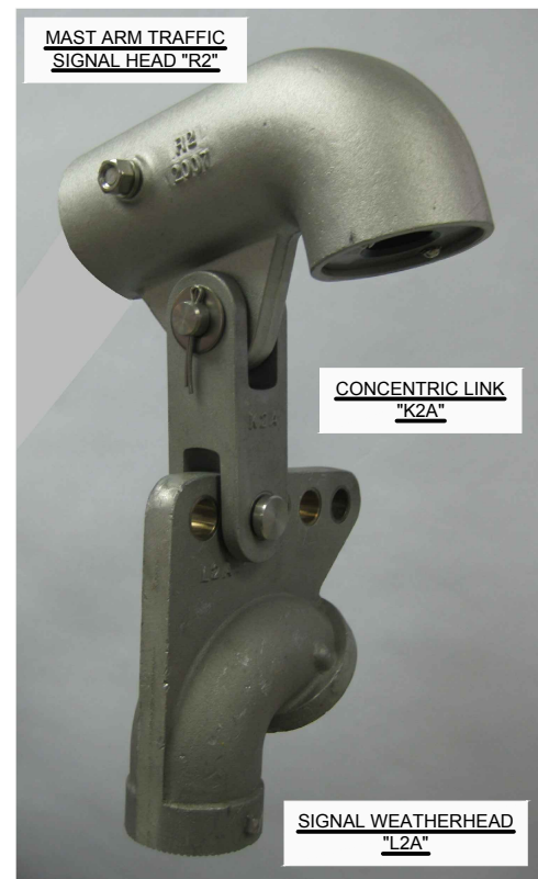
"MAW-15" SIGNAL SUSPENSION ASSEMBLY
