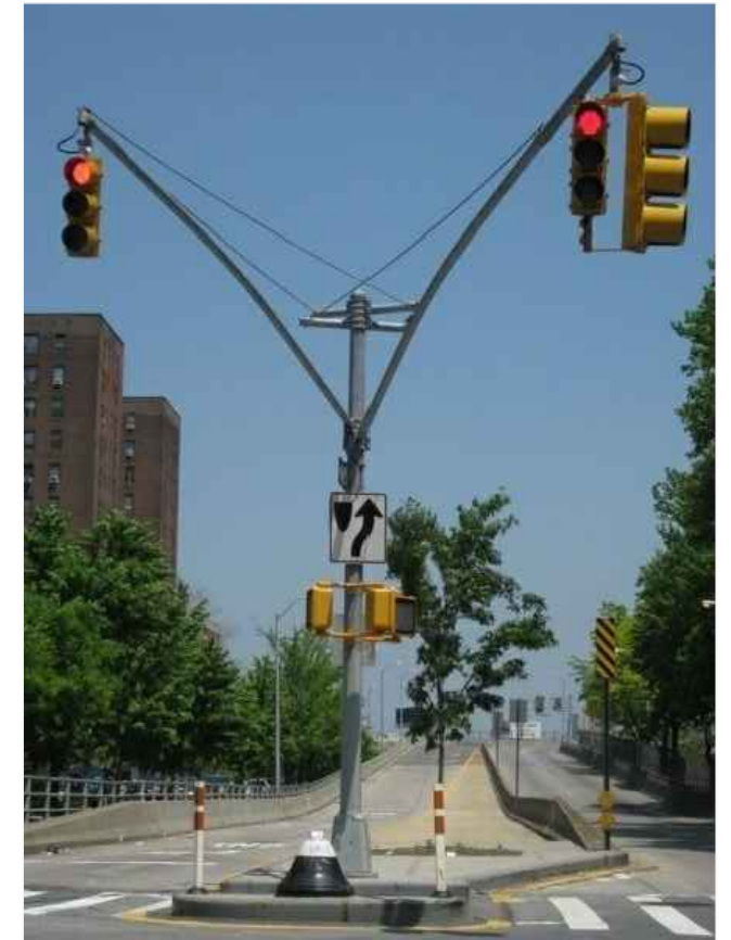
DOUBLE ARM TRAFFIC SIGNALS ON "M-2A" POLE
