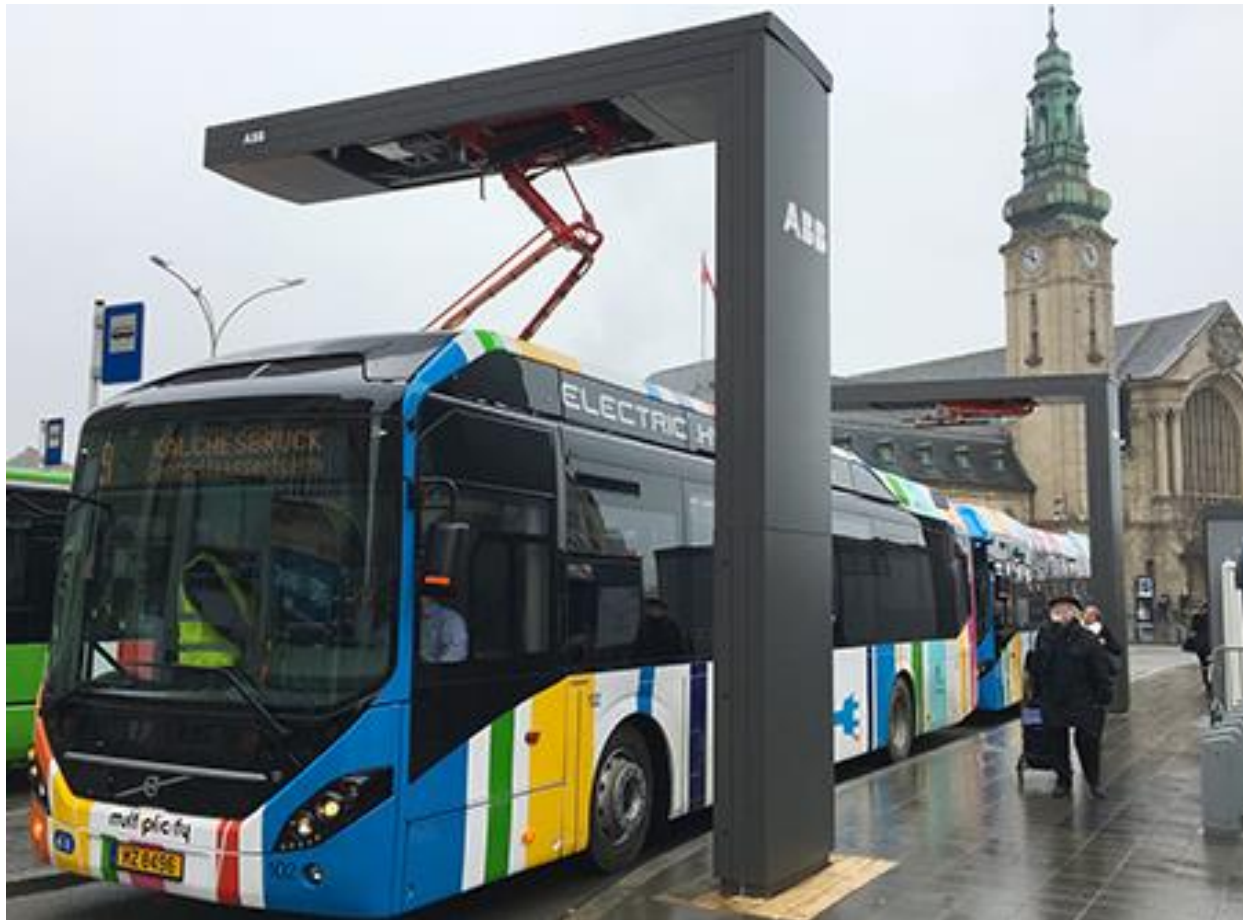
Figure 41 Automatic electric bus charging stations, 600kW max capacity (source: ABB)
