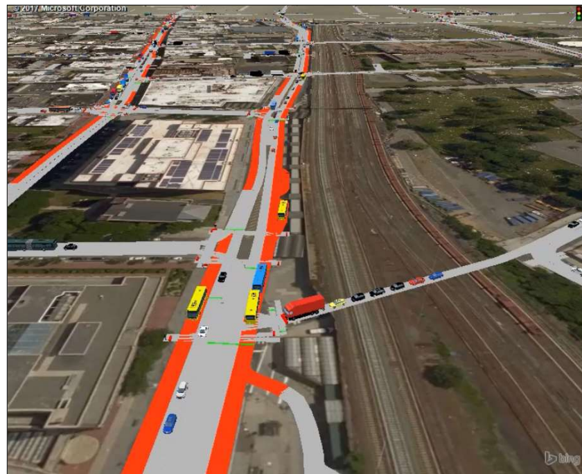
Figure 4-15: Snapshot of VISSIM Analysis at Archer Avenue/153rd Street - Existing Conditions PM Peak Hour
