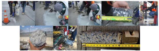
Removing a Core from 252<sup>nd</sup> Street Bridge over Henry Hudson Parkway in January 2009. (Credit: Masroor Mahmood) Core Sampling on the Bay Ridge Avenue Bridge in 2014. Utilizing a Coring Machine to Obtain a Concrete Core for Testing in June 2016 from the Westbound BQE over Adams Street.
