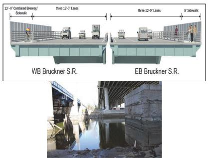
Proposed Bridge Cross Section. Area of Bridge Widening.
