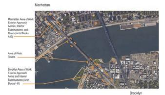
The Manhattan Approach is a continuous arch masonry structure consisting of brick, granite, limestone and infill concrete. The arches run between the Manhattan Anchorage at the east and
