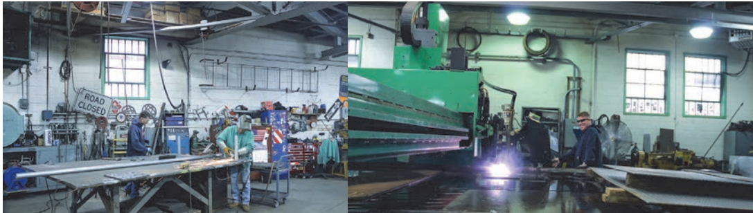
May 2017: Bridge Repairer and Riveters Daniel Wynne, Charlie Zhao, and Randall Palmenta Demonstrating Welding Steel and Cutting With a Plasma Machine. (Credit: Samuel Teaw)
