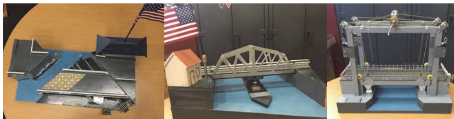
Working Models of Rolling Lift Bascule, Retractable, Swing, and Vertical Lift Bridges created by Machinist Mark Blokh in 2016. (Credit: Vera Ovetskaya)
