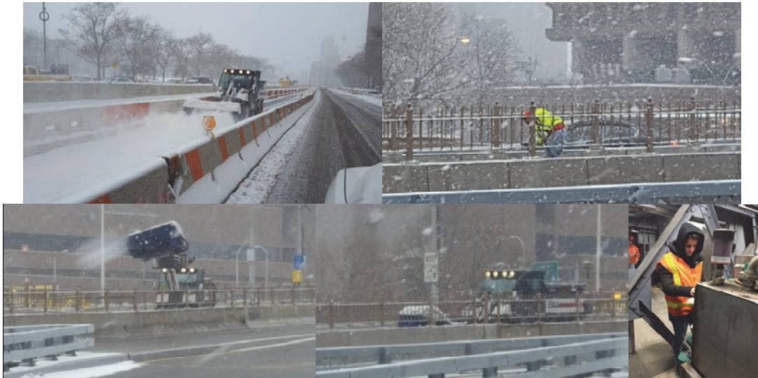
January 2017: New Toolcat With Front Brush Attachment Clearing Snow From the Brooklyn Bridge Bicycle/Pedestrian Path. Shoveling Snow by Hand. Bobcat Vehicle With Broom Attachment Raised up High and Lowered. There Are Some Narrow Passages Along The Pathway That Cannot be Accessed by the Broom, so These Areas are Cleared by Hand. The Bobcat Passes These Areas With the Broom Raised. (Credit: Paul Schwartz) March 2017: Assistant Mechanical Engineer Nazariy Davydovych Checking the Temperature of the Hydraulic Fluid on the 145 th Street Bridge. (Credit: Vera Ovetskaya)
