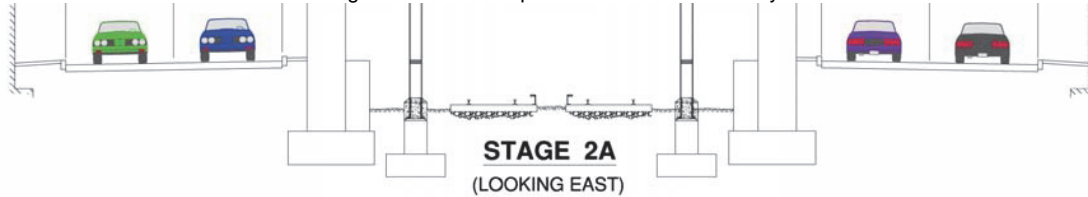
Stage 2A - Remove/Replace Eastbound Roadway.
