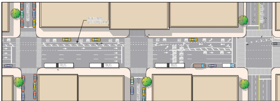
Figure 3.8.3: Bike Lane on 8 th Avenue in front of PABT.
