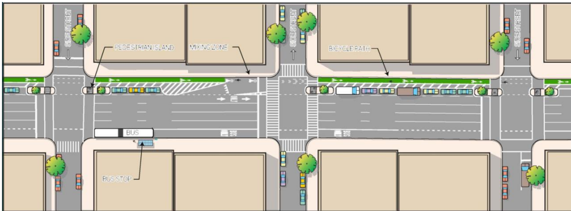
Figure 3.8.1: Typical Plan for 8 th and 9 th Avenue Bike Lanes with Mixing Zones at Minor Cross Streets.
